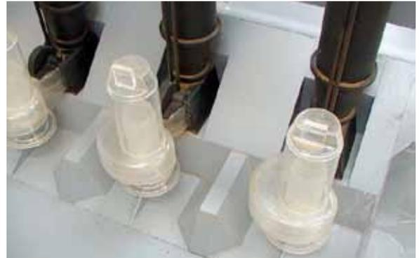
Centrifugal pump sump design verified by a scale model test.
